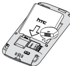
2. With the exposed side of the back cover facing up, insert the top part of the phone into the back cover.
